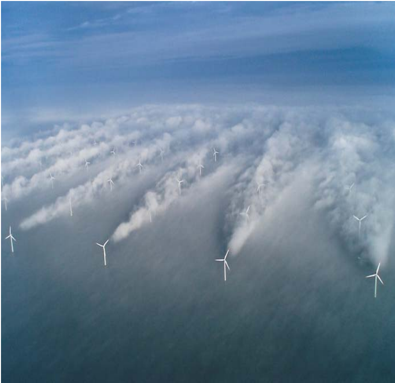
Fig. 7 Cloud formation in a wind farm in high humidity air. The turbulence behind the turbines leads to nucleation of water droplets. The condensation releases the large latent heat of the vapor to fluid phase transition to the atmosphere. The size of the formed cloud indicates the level of atmospheric heating by the wind turbines.
